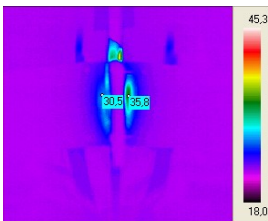
Fig.1 Thermogram of nonwoven without PCM at 355 second of heating
